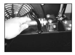
Figure 14: Connecting Water Hose
